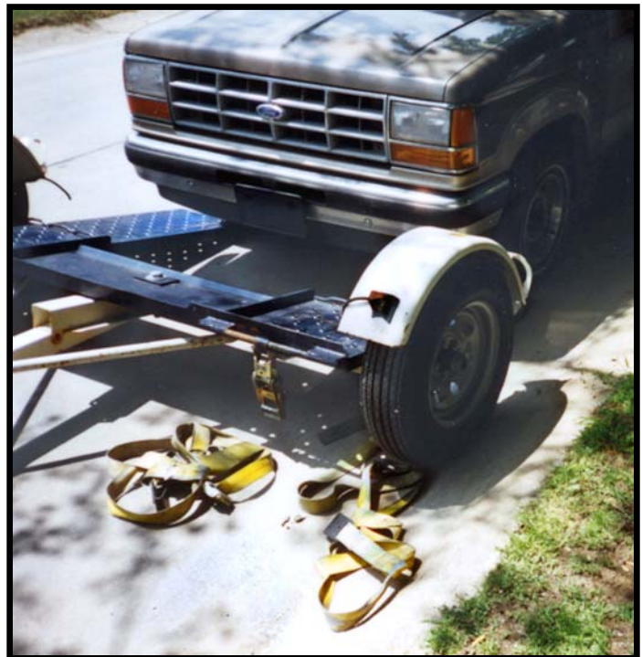
Photo 2 – Closer view of the dolly showing hold-down straps on the ground and position of the vehicle-in-tow.
