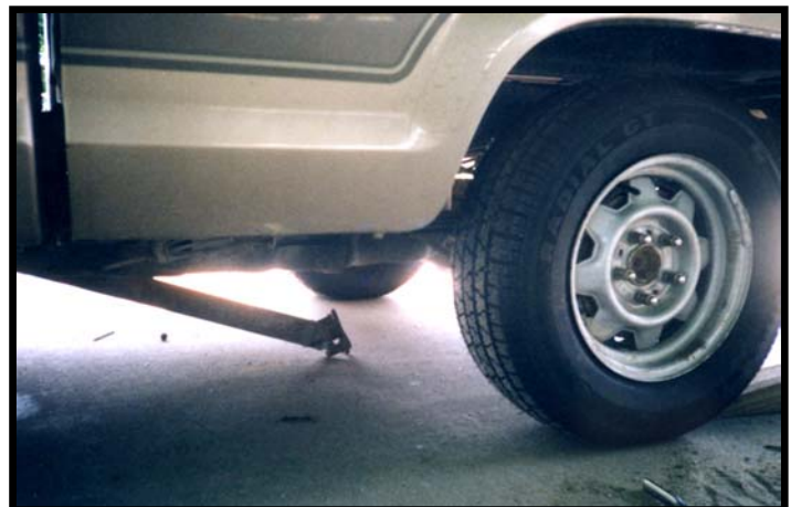
Photo 4 – View from driver's side of the vehicle-in-tow showing the driveshaft disconnected from the differential.
