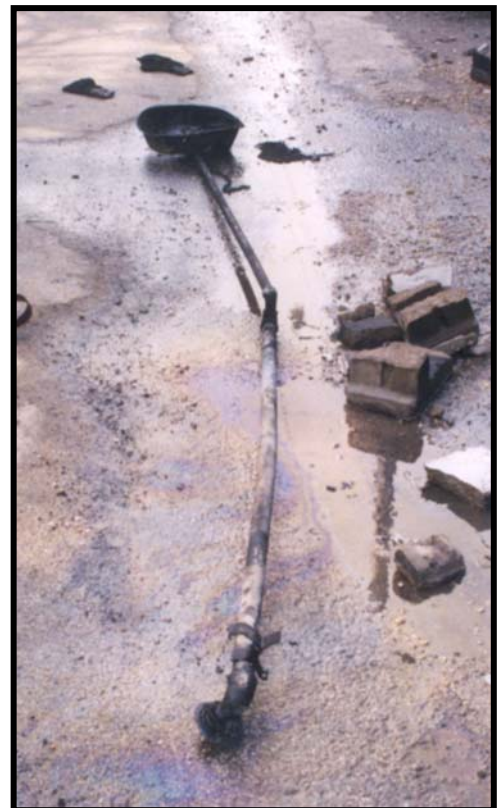
Photo 2 – Articulated pipe with oil pan on one end, and broken fitting for the oil barrel on the other.
