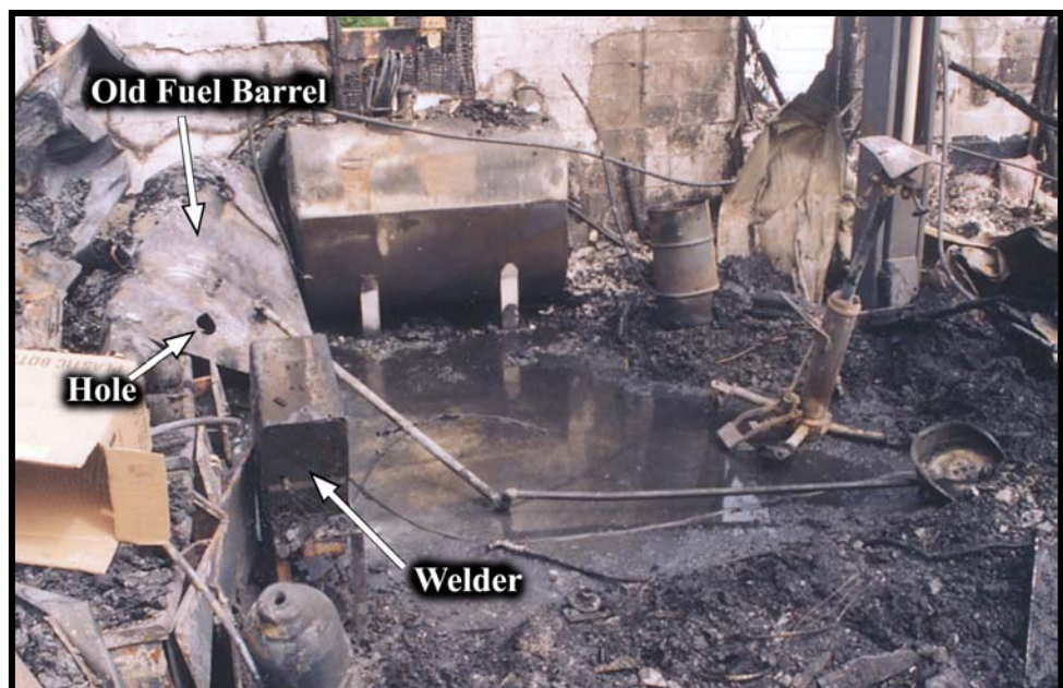
Photo 1 – View of the burned out shop area, showing the old fuel barrel and welder.
