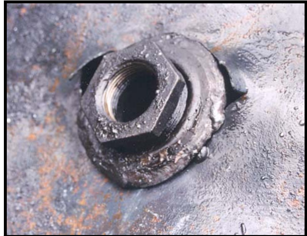
Photo 3 – Close-up of bung hole showing broken welds that were being repaired.
