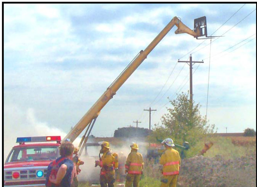
Photo 1 – View of firefighters at the scene, showing the forklift near the powerlines and the pump suspended by a wire rope cable.
