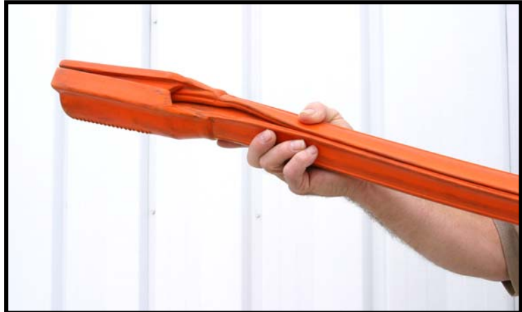
Photo 5 – Rubber sleeve (guts) used to insulate powerlines.
