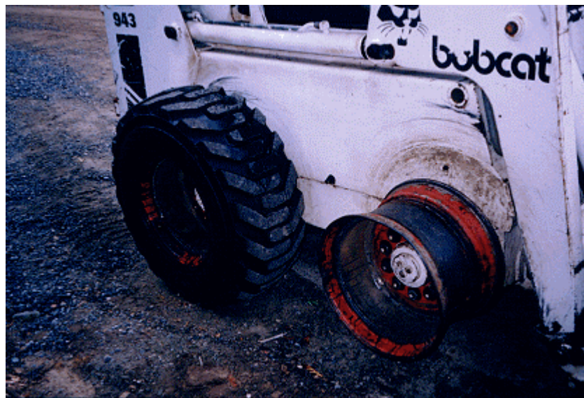
Figure 2. Rim wheel of the skid-steer loader after the explosion.
