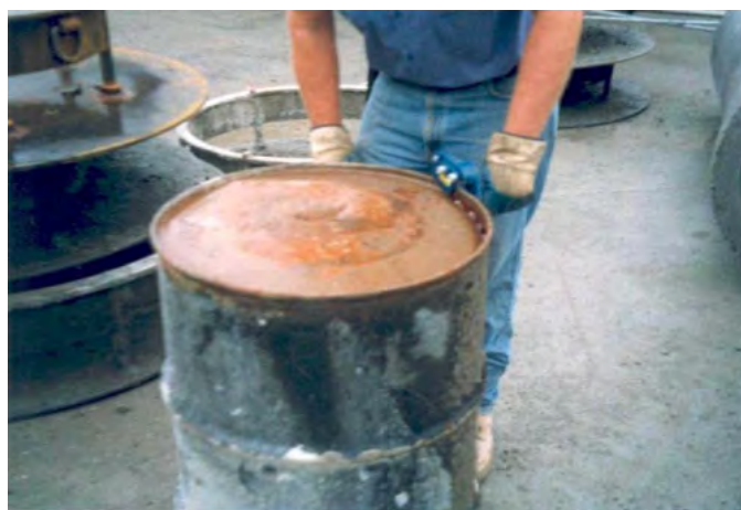
Figure 1 – Employee using hand held drum opener to open a 55-gallon drum.
