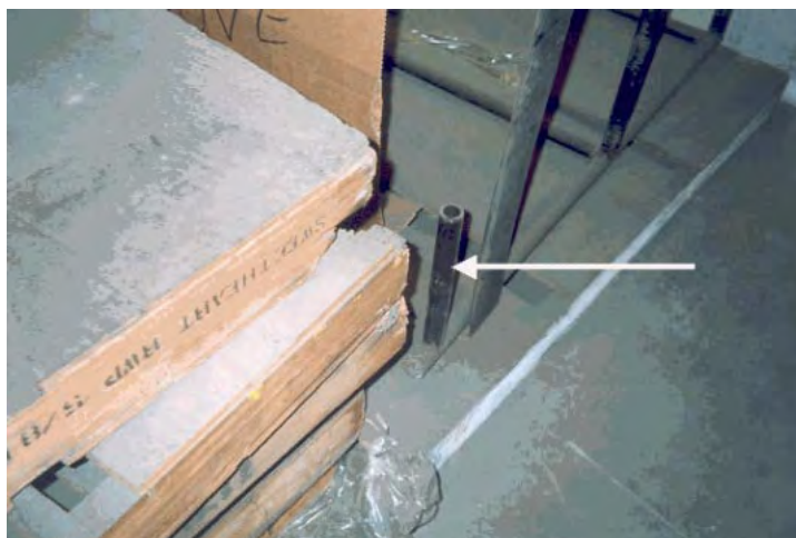
Figure 5 – L-shaped metal tubing that slid into the same opening in the pallet as the order picker tines connecting the guardrail to the pallet.
