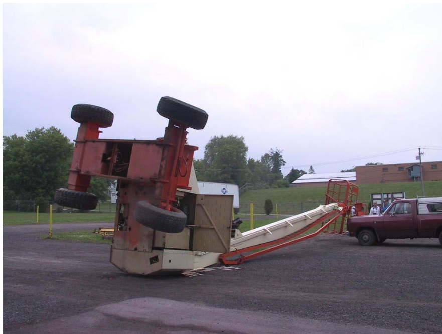
Figure 2. The aerial work platform tipped over during the incident and hit a pickup truck that was parked near by.
