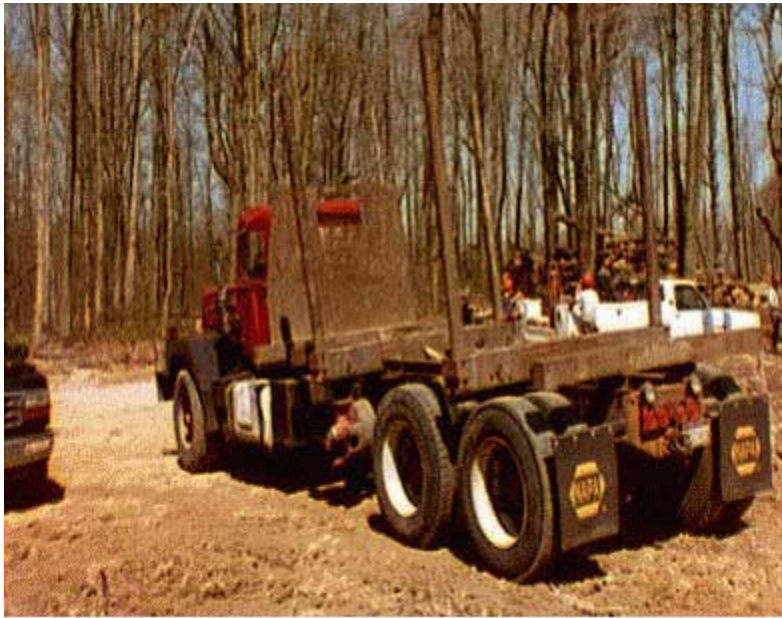
Figure : The above photograph shows the truck involved in the fatal incident. At the time of the incident, the load extended approximately one foot above the standards. Although this is not the exact location of the incident, the final relationship between the truck, victim, and fatal energy source are represented.
