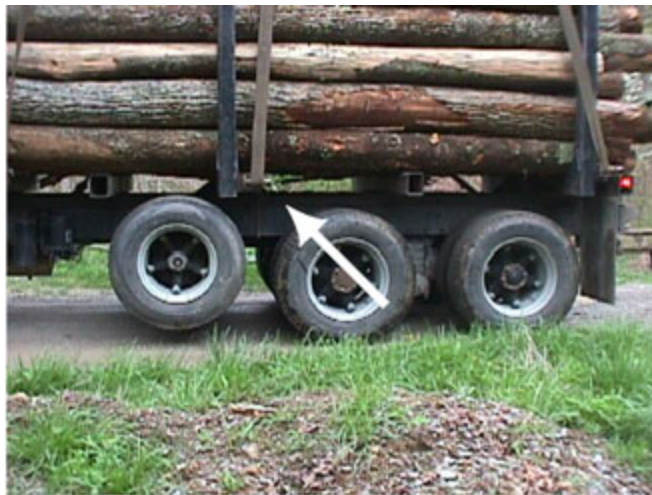
Figure 3. Arrow indicates binder being accessed when log struck victim.
