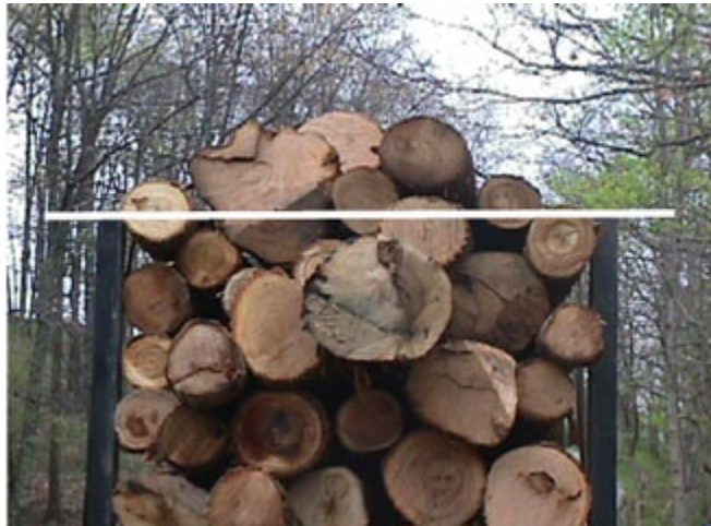
Figure 6. This is the rear view of the same truck loaded the day of the investigation. White line represents the plane created by the top of the standards. Note the height of logs above the line.
