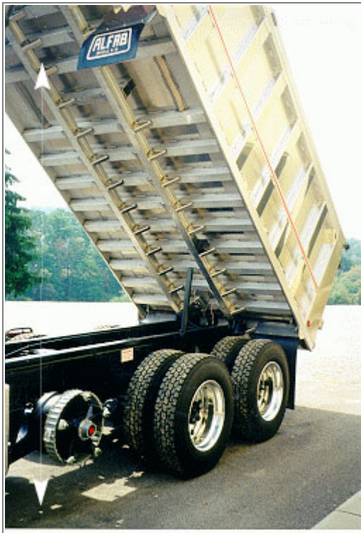
Distance of the end pin mountings when body prop is used
