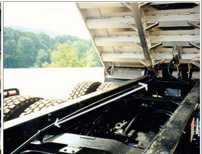
Pull-off cable running along the truck's frame
