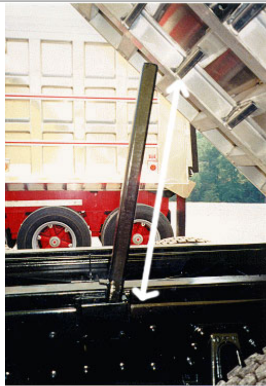
Close-up of the safety body prop when body is in an elevated position
