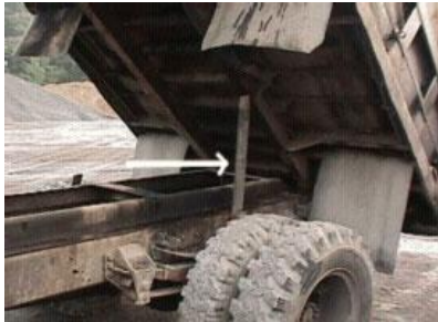
Figure 4. The arrow points to the convenient and permanently attached body support installed after the incident as per OSHA's recommendations. The support folds when not in use.
