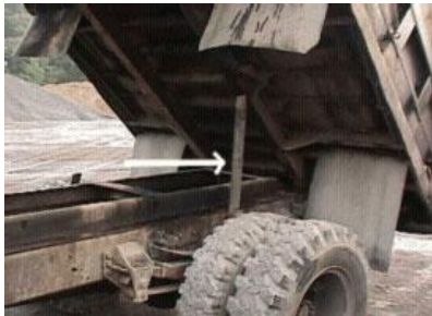
Figure 5. This photo shows the center section of the stretched and unprotected cable.
