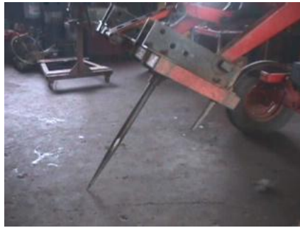
Figure 2. Factory installed end-loader attachment and after market bale spike.
