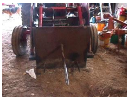
Figure 2. Front end-loader attachment and fabricated bale spear.
