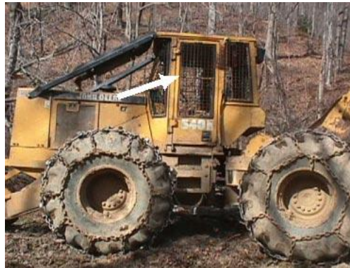
Figure 1. This is the skidder which ran over the victim. The arrow points to one of two doors which were not present the day of the incident.
