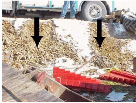
Figure 4. The black arrows indicate the slide marks which were made by the front left and rear wheels. The point of the arrows indicate the approximate position of the wheels when the tractor began to roll. This photo was taken over the bottom of the overturned tractor. In the foreground is the end loader bucket. From this perspective, the front of the tractor is on your left.
