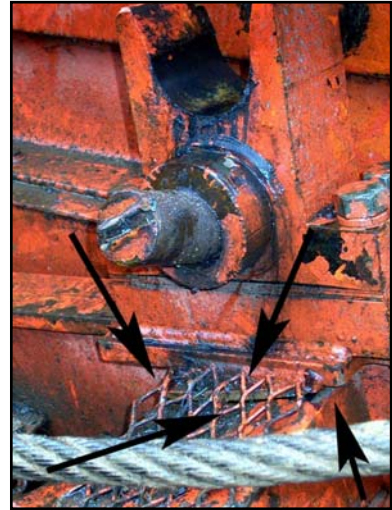
Tower hinge and box beam (arrows) broke, allowing tower to come down.
