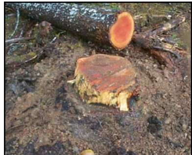
Anchor stump #2. Fresh dirt indicates the stump pulled out of the ground and released its guyline.
