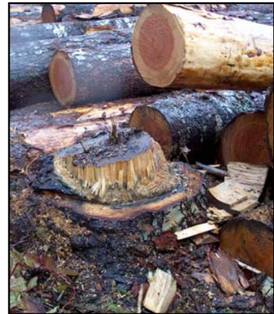
Anchor stump #1. The cable pulled over the top of the stump. Note proximity of log deck to stump (see Recommendation #1).
