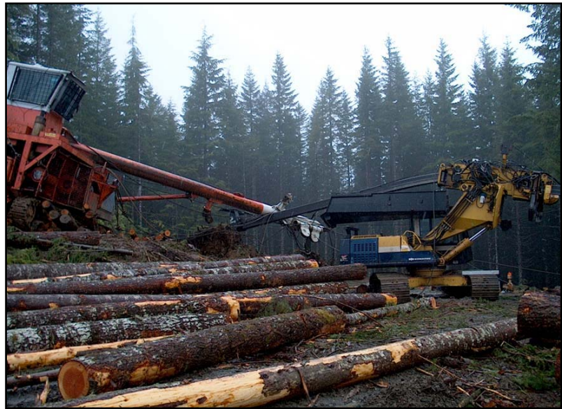
When guyline support failed, the yarder tower fell onto a nearby delimber (right).
