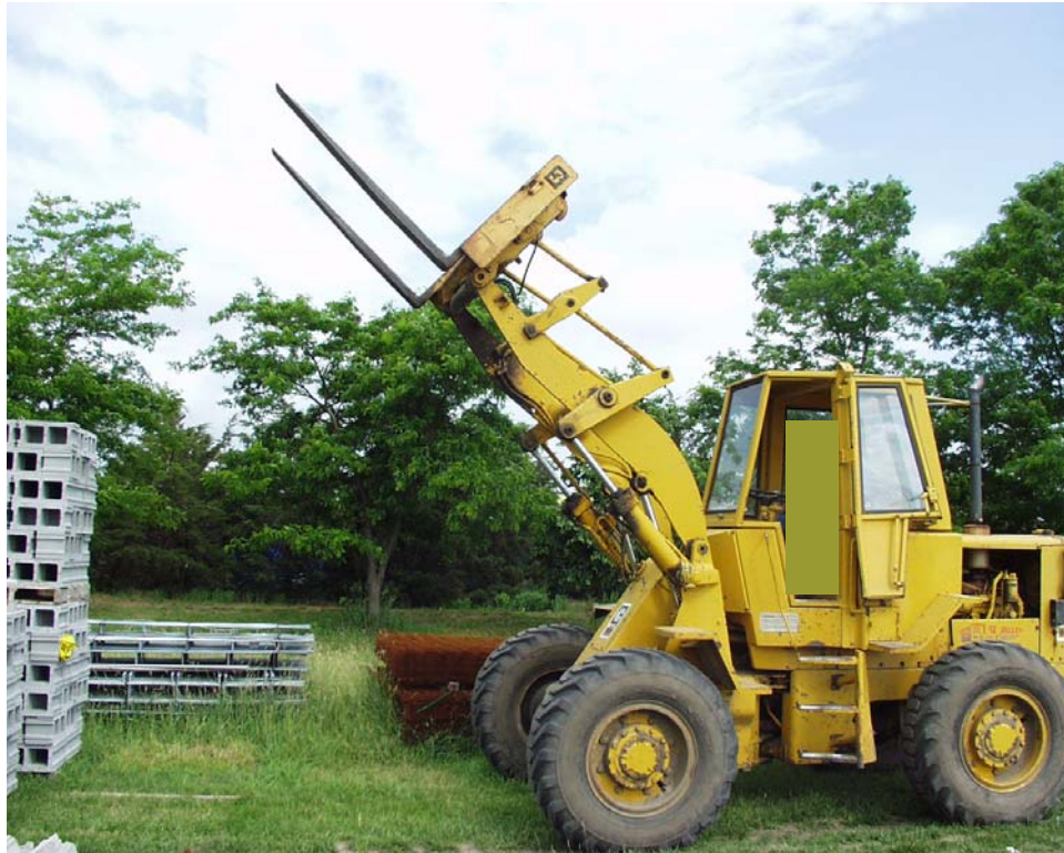
Incident forklift in the maximum raised position necessary to clear concrete blocks.
