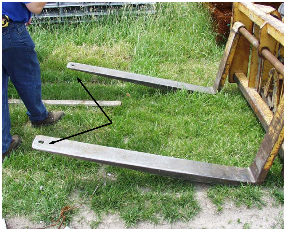
Arrows indicate holes cut into forklift tines.
