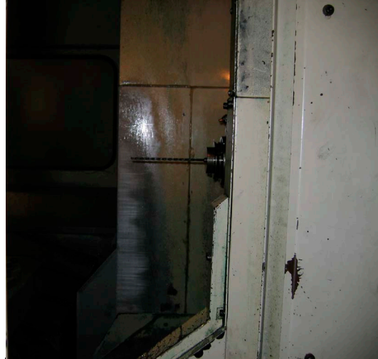
Figure 2. Example of tool in holder within the CNC machine with doors open
