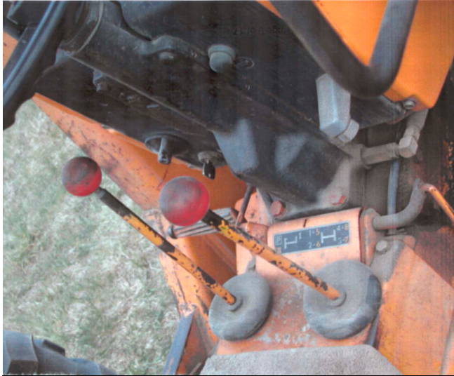
Figure 4. Position of gear levers taken after incident.
