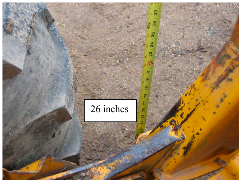
Figure 2. Height of subframe from ground
