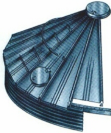
Figure1. Typical Steel Bin Roof with Access Hatch and Center Opening Cover
