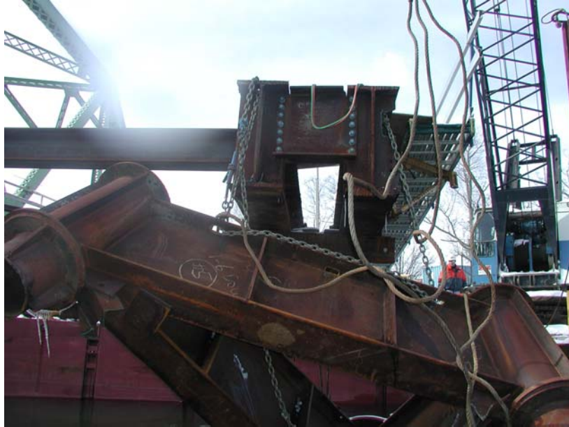
Photo 5. The pile cap hung by the test chains after it broke apart from the W36 I-beams.
