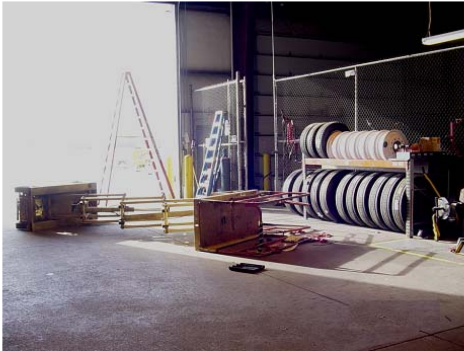
Photo 2. Post incident scene: the scissors lift was struck by the garage door after the door was released by the victim, toppling the lift. (Courtesy of OSHA)
