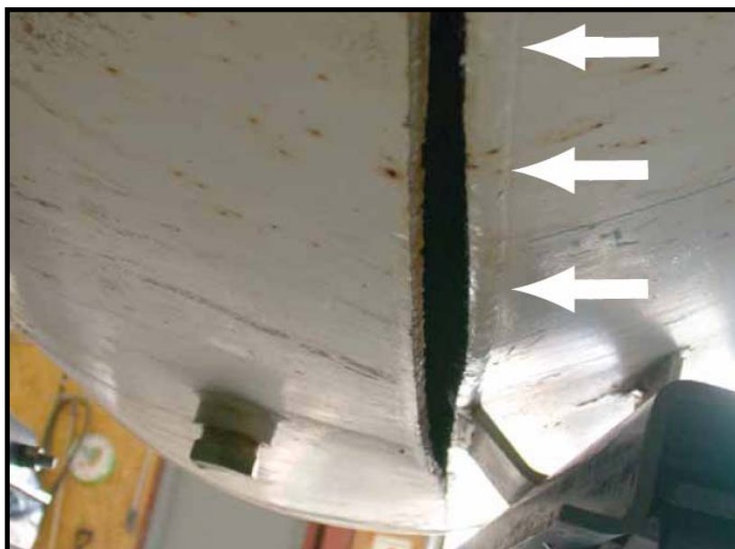
Photo 2 – The underside of the nurse tank with close-up view of fracture site. (Photograph courtesy of NTSB)
