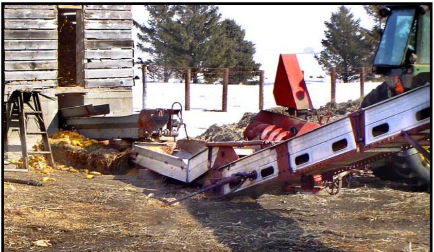
Photo 1 – Overview photograph of the area, showing the east end of the corn crib, the chain drag conveyor, and the flight elevator with half of the PTO driveshaft attached.
