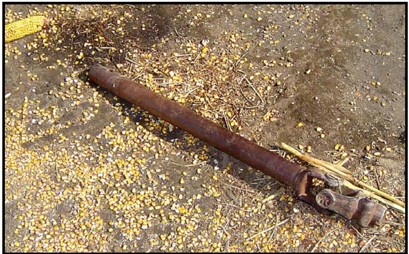
Photo 3 – Tractor end of PTO driveline, with no evidence of shielding.
