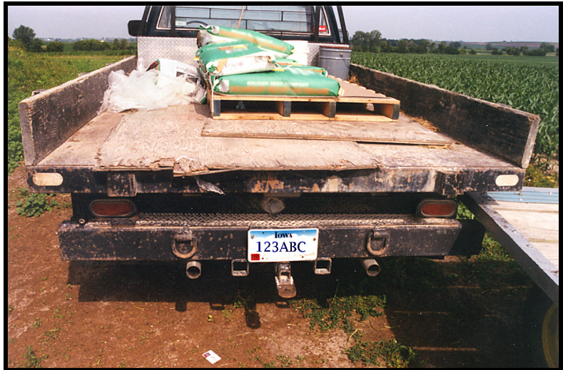
Photo 3 – View of rear of truck showing relative position of bumper and truck bed. Hay wagon shown to the right is typical, but is not the one involved in this incident.
