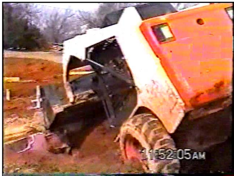
Figure 3. Skid-steer loader tipped forward (from video filmed after the incident)
