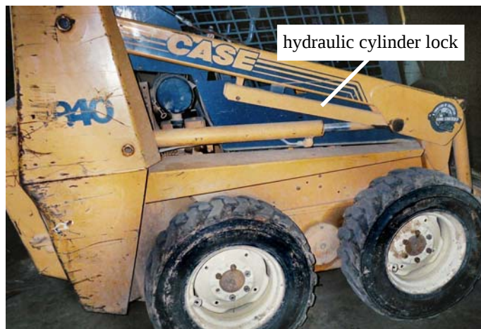
Photo 4 - Hydraulic cylinder lock in stowed position.
