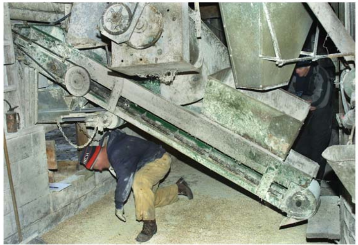
Photo 5 and 6 - Shows the height and location of the rotating shaft. Photo 6 shows how the farmer had to routinely duck under the conveyor from side to side to access the switch panel.
