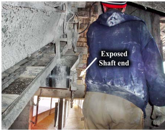
Photo 5 and 6 - Shows the height and location of the rotating shaft. Photo 6 shows how the farmer had to routinely duck under the conveyor from side to side to access the switch panel.
