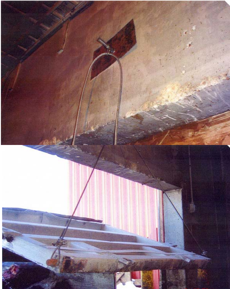
Figure 4. The semi trailer gate maintained in a raised position by the wire sling attached to the semi trailer locking pin and the attachment point above the door.
