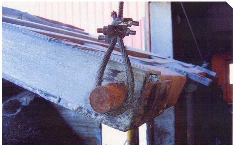
Figure 2. The locking pin and wire sling on the semi trailer gate.
