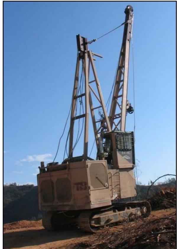
View of a yarder in transit to a new location at a logging site.
