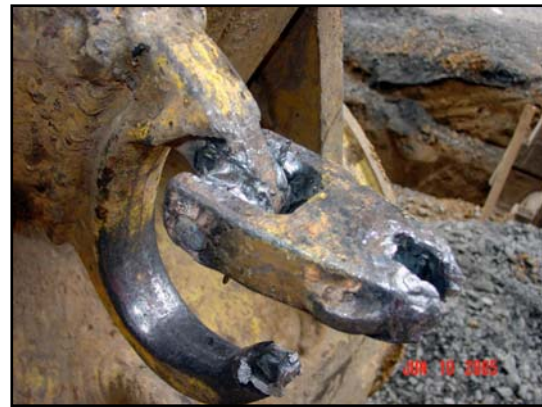
Part of the latch remained attached to the hook welded on the Hendrix Quick Coupler on the arm of the track-hoe.
