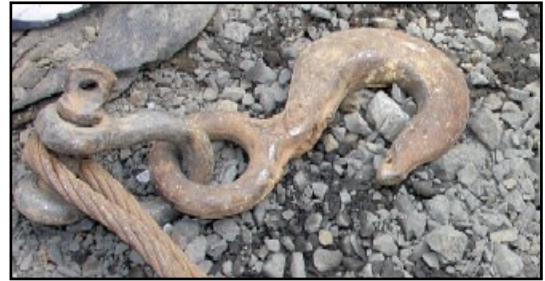
The hook and shackle attached to the track-hoe, like the one shown here (without the cable), snapped loose when the rigging failed and struck the pipelayer.
