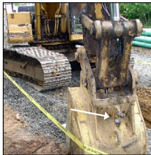
latched hook welded onto the quick-coupler to replace the original closed "lifting eye" supplied by the manufacturer.
