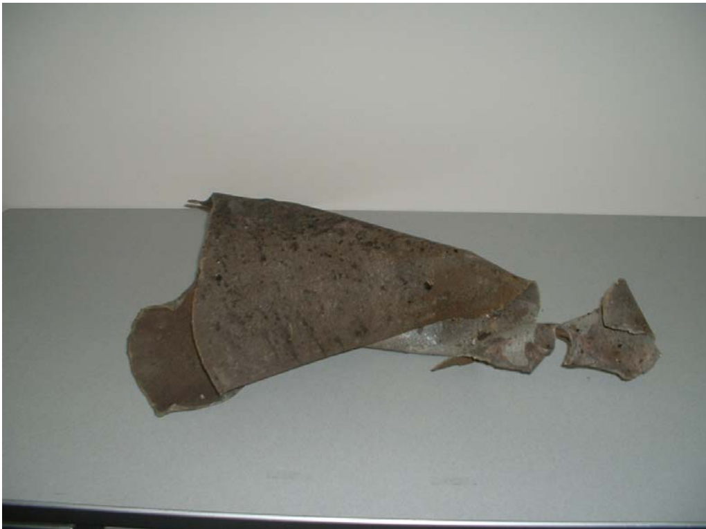
Exhibit 6. A piece of the exploded tank showing the inner wall and oily substance
