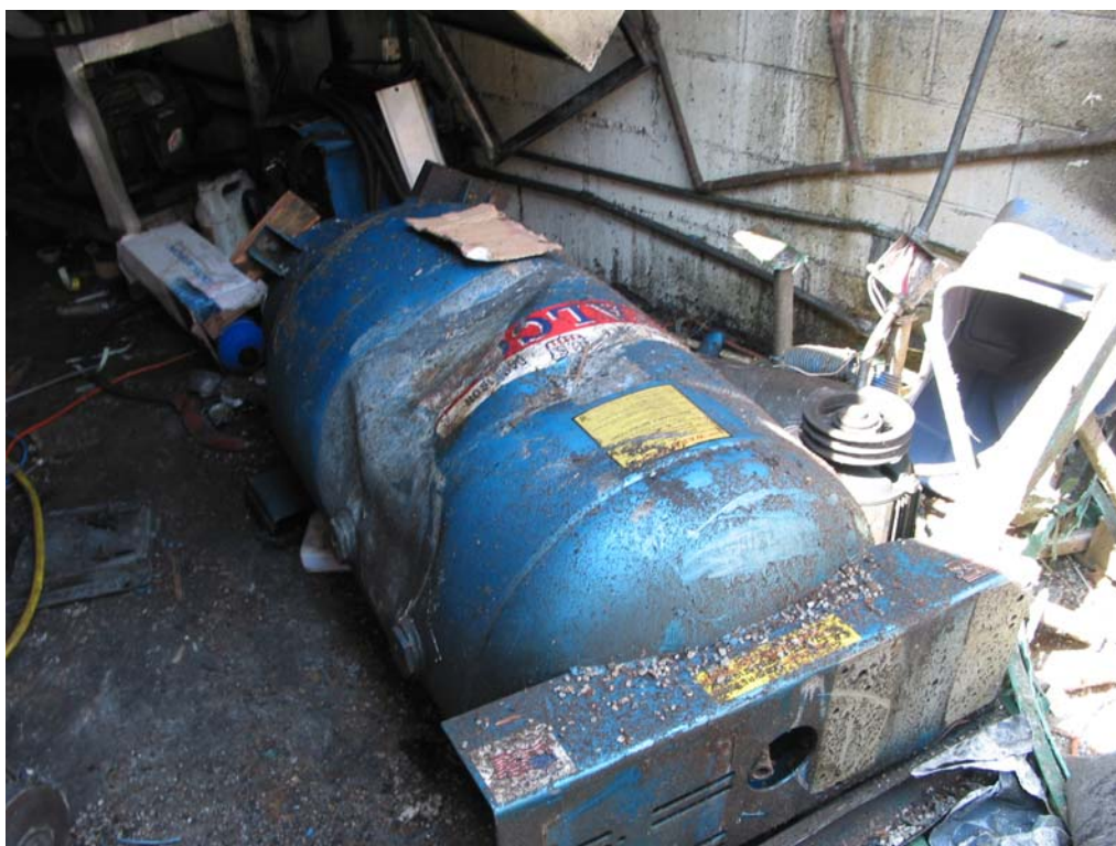
Exhibit 4. The second air tank inside the equipment room, which did not explode.
