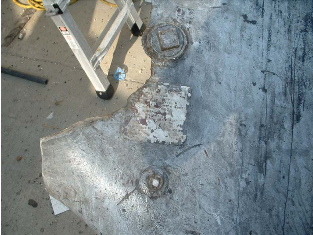
Exhibit 5. A piece of the exploded tank
