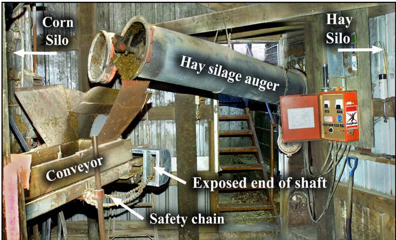
Photo 3 - Composite photograph from the west end of the shed showing both silos, the end of the conveyor belt (now with guard), and the control panel for the hay silo.
