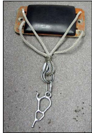
Detail of a boatswain's chair shows attachment to a descender with a screw-type carabiner.
