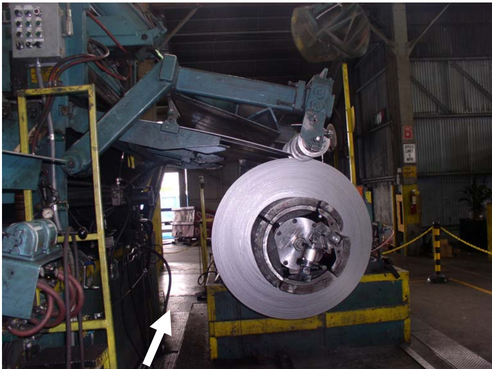
Exhibit 3. A picture of the rewind cylinder from the side showing where the victim was standing (white arrow) prior to getting entangled in the steel.
