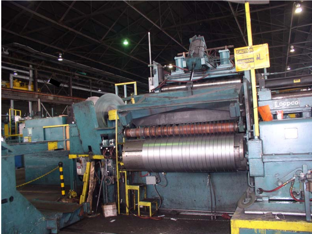
Exhibit 2. A picture of the rewind cylinder with the cut steel being wound onto the cylinder.
