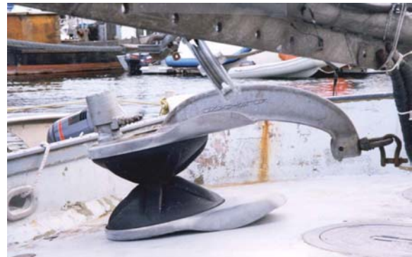
Figure 4b. Power block
