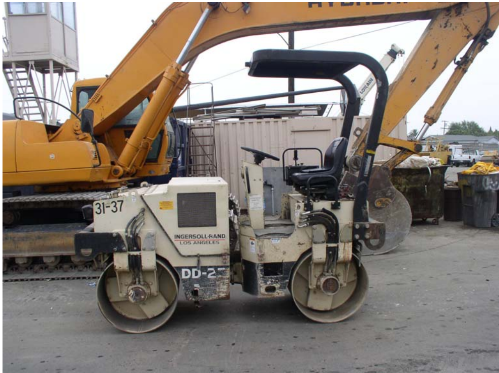
Exhibit 1. A picture of the articulating vibratory tandem-drum compactor roller involved in the incident.
