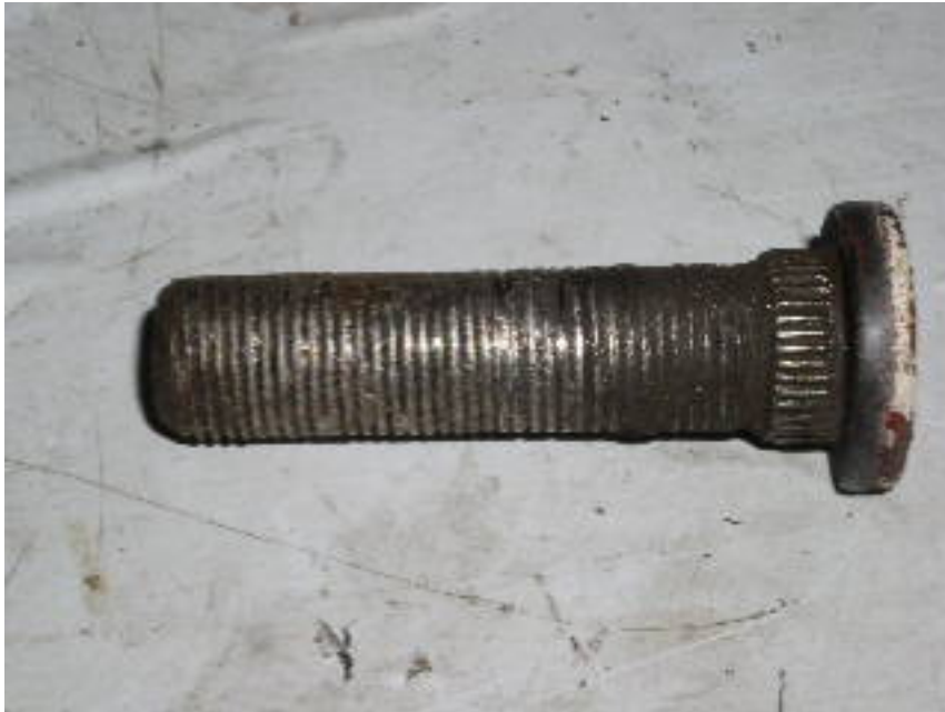
Exhibit 3: A picture of a wheel stud involved in the incident showing all the threads flattened by the explosion.
