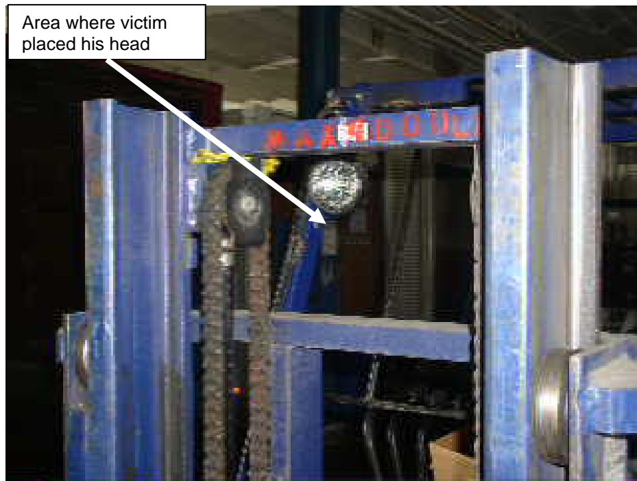
Exhibit #2: A picture of the forklift mast showing where the victim placed his head.
