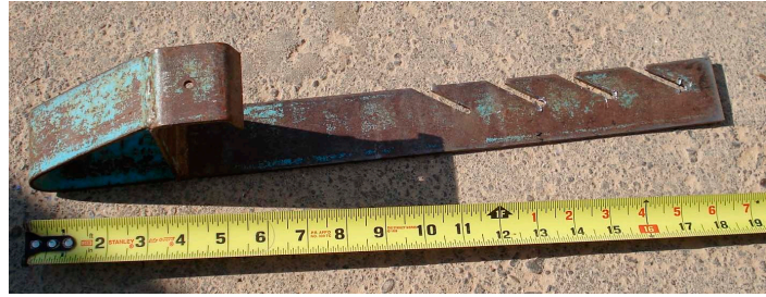
Figure 4. Roof bracket similar to type decedent installed
