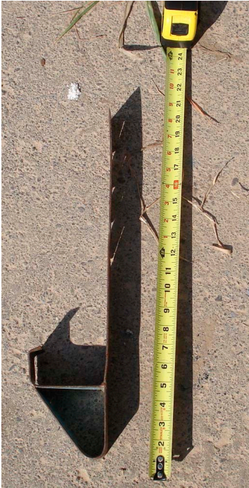
Figure 3. Roof bracket similar to one decedent installed
