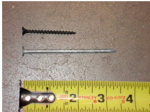
Figure 5. 2-inch drywall screw used by decedent compared to 16d nail.
