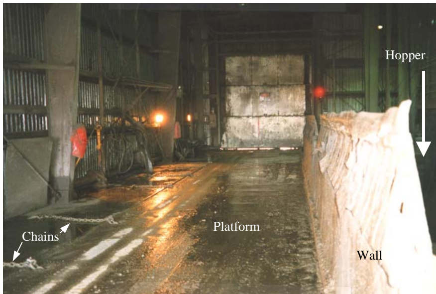
Figure 2b. Dumping platform and wall adjacent to hopper
