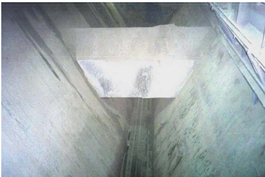
Figure 3. Hopper, center divider, and conveyor belt at bottom
