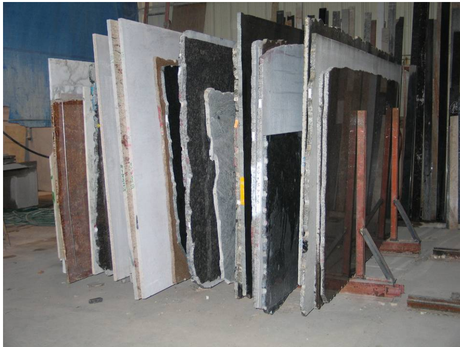
Figure 1 – Slab rack involved in the incident (end support pins had been welded to the rack by the company)
