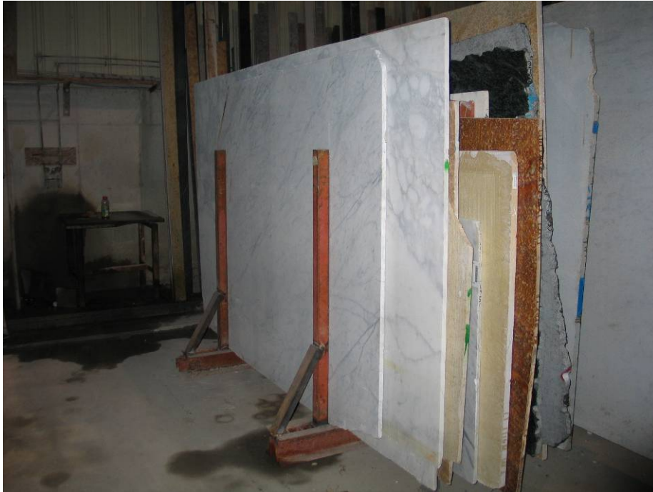
Figure 2 – At time of the incident the end support pins were removed.
