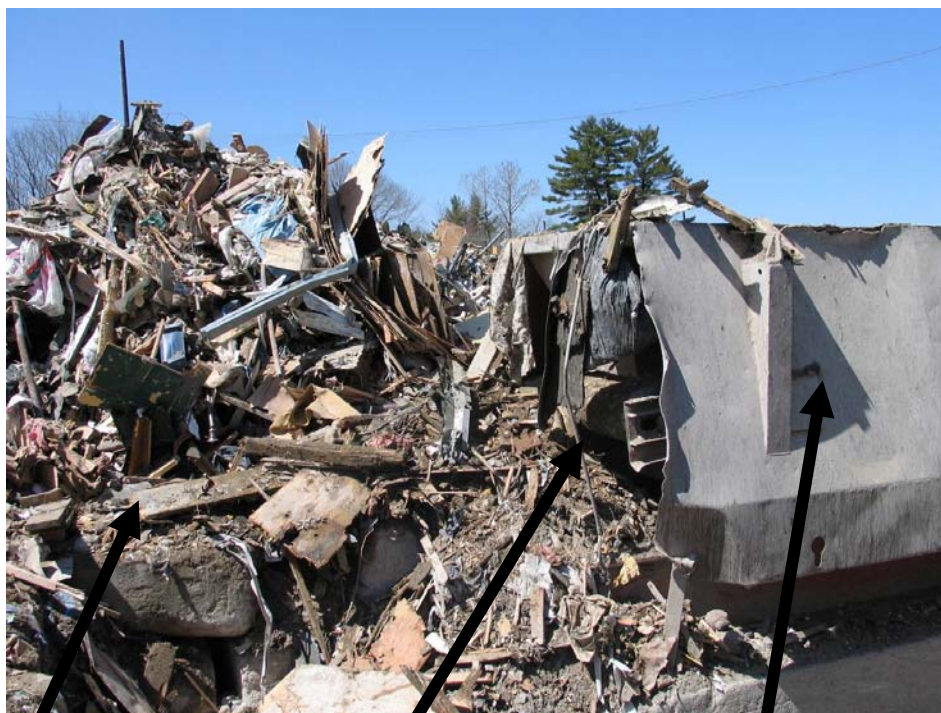
Figure 2 – Debris pile, system's conveyor belt and hopper, and incident location
