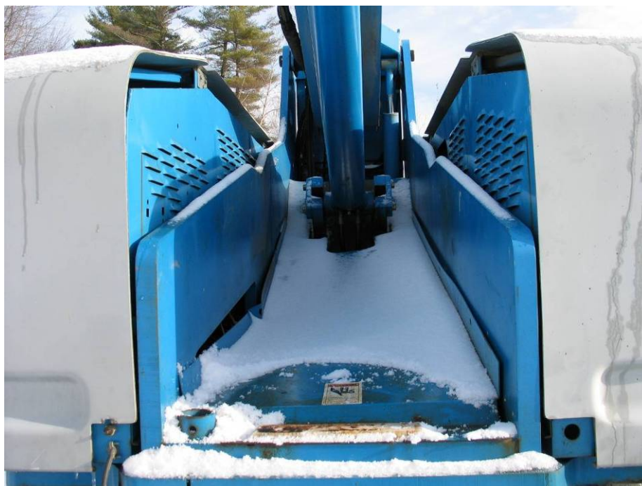
Figure 3 – Location where victim was crushed and a decal warning of a crushing hazard.
