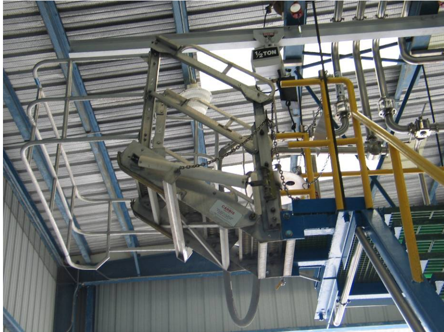
Figure 2 – Platform system's gangway that the victim fell from in the stored position.
