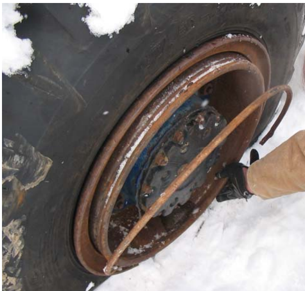
Photo 6. The dislodged lock ring was being refitted to the multi-piece wheel that was involved in the incident (Photo courtesy of OSHA).
