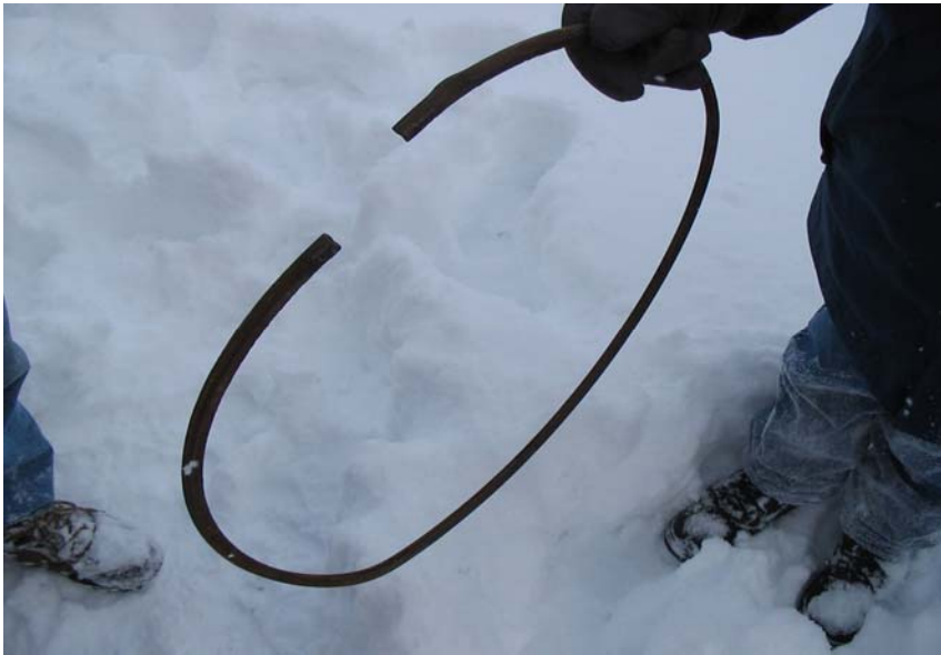
Photo 5. The lock ring that was propelled from the multi-piece rim wheel; it struck the victim while he was inflating the rim wheel (Photo courtesy of OSHA).
