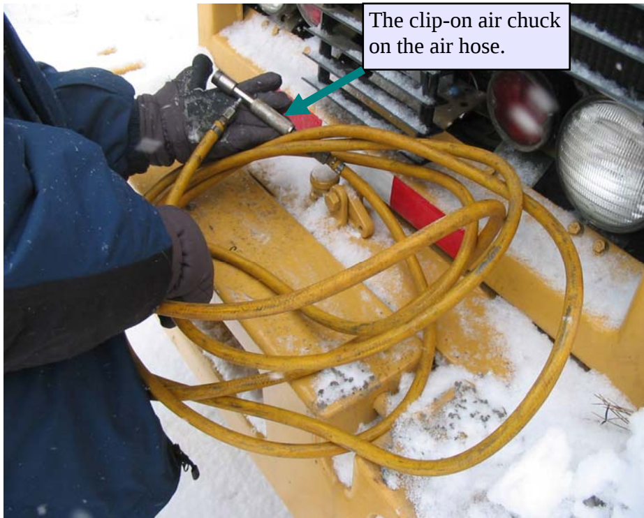
Photo 3. The air hose that was used by the victim and the co-worker during the incident. The hose had a clip-on chuck on one end. It did not have an in-line gauge (Photo courtesy of OSHA).
