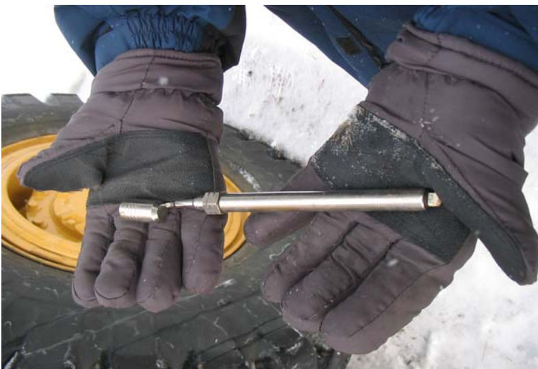
Photo 4. The hand-held air pressure gauge used by the victim during the incident (Photo courtesy of OHSA).
