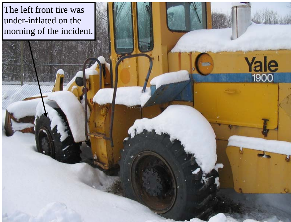
Photo 2. The loader that was operated by the victim on the morning of the incident. The left front tire was under-inflated at the time of the incident. (Photo courtesy of OHSA)
