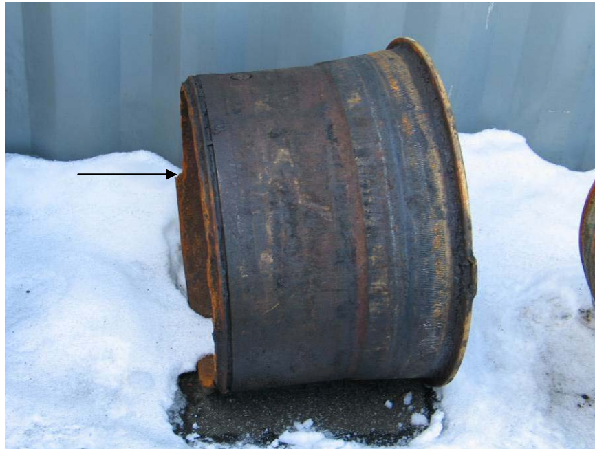
Figure 4 – Rim component of the multi-piece rim wheel that failed. The arrow is pointing to the section of the rim component that cracked and failed.
