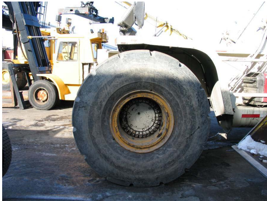
Figure 3 – Container handler with replaced wheel.
