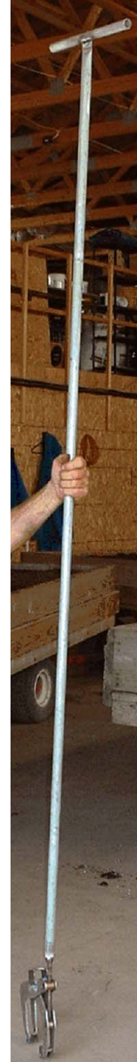
Figure 7. Tool developed to add/remove stop logs
