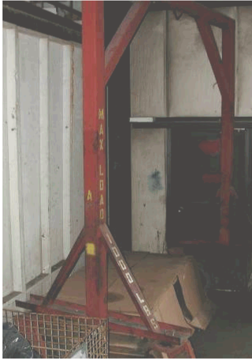
Photo 5. The gantry crane was raised with the addition of wheels and tires. This also raised the center of mass of the crane.
