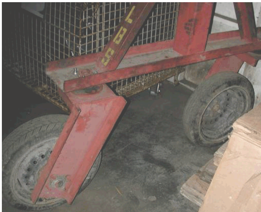
Photo 6. Vehicle wheels and tires were attached to the gantry crane at the ends of the horizontal bars. The wheels all rotated 360 degrees and were not coordinated to turn together.
