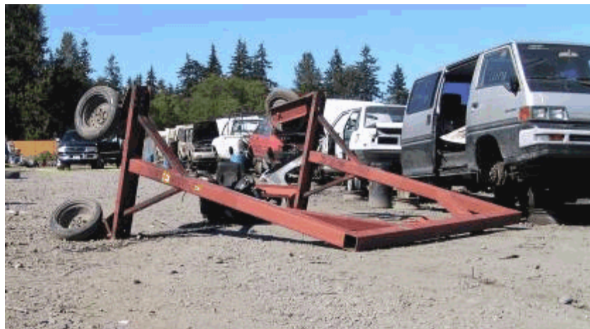
Photo 2. The incident site showing the gantry crane in the final resting position and the engine and transmission situated between the wheels. Notice the uneven gravel surface with large rocks and depression obstacles.
