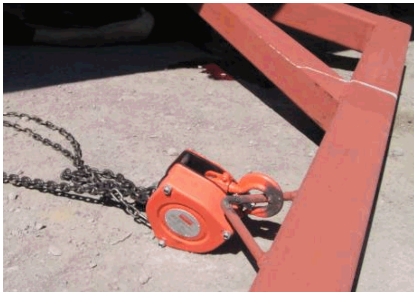
Photo 4. The manual chain pulley was able to swing freely at attachment point and allowed suspended loads to move freely.
