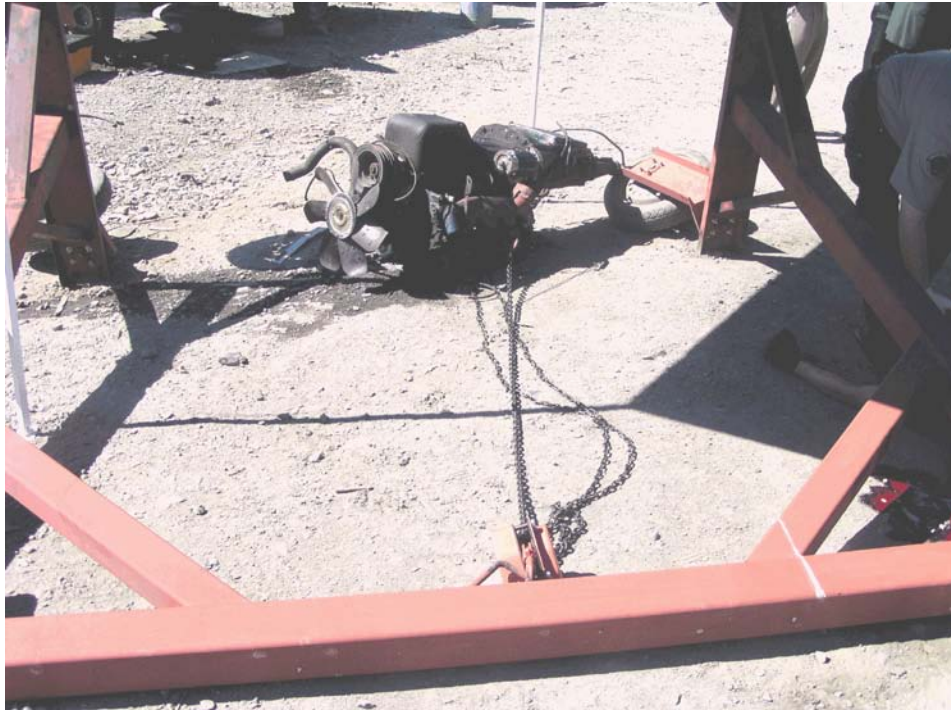
Photo 3. The engine and transmission were attached to the gantry crane with a manual chain pulley. Notice the lack of lines or attachments that could have been used to stabilize the load and prevent it from swinging.
