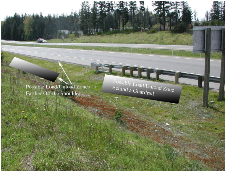
Photo 4: This figure shows several additional options, just beyond the site of the incident, for parking a trailer to load/unload that might provide better protection than the shoulder.
